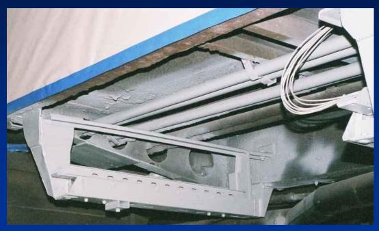
Lower rail nests in structural channel – separated by rubber vibration dampeners
